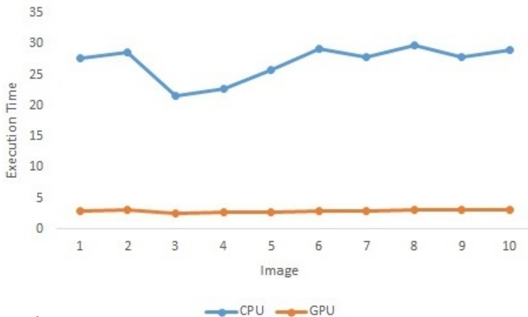
Figure 5.1: Execution time of serial algorithm on CPU and parallel algorithm on GPU
