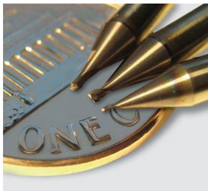
Figure 4.1: Micro end mills
