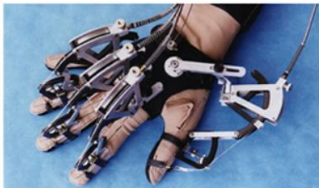
Figure 1.1: glove based hand gesture[34].
