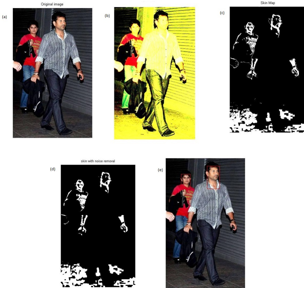
Figure 3.4: Example-1 : (a) original image, (b) input image in YCbCr color space, (c) brightness compensated image of the input image, (d) skin map of input image, (e) skin map of input image after noise removal, (f) Final output image with the detected faces
