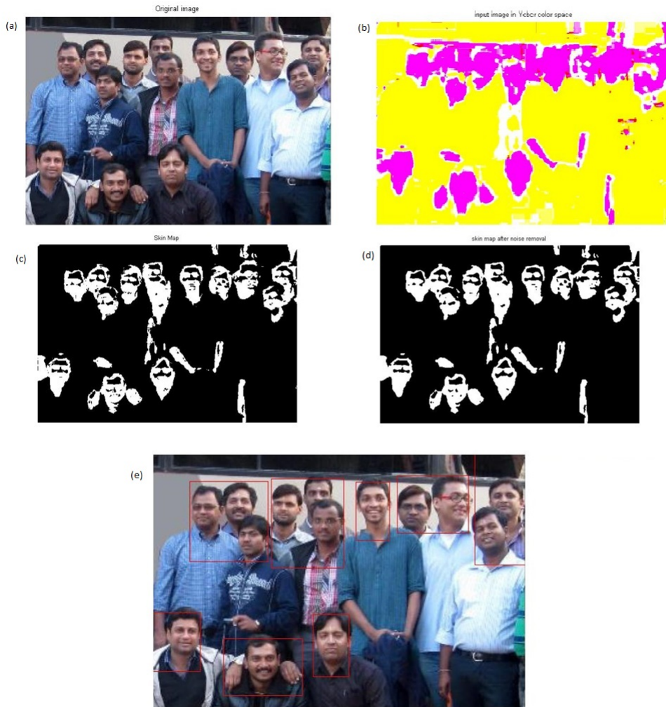
Figure 3.5: Example-2 : (a) original image, (b) input image in YCbCr color space, (c) brightness compensated image of the input image, (d) skin map of input image, (e) skin map of input image after noise removal, (f) Final output image with the detected faces
