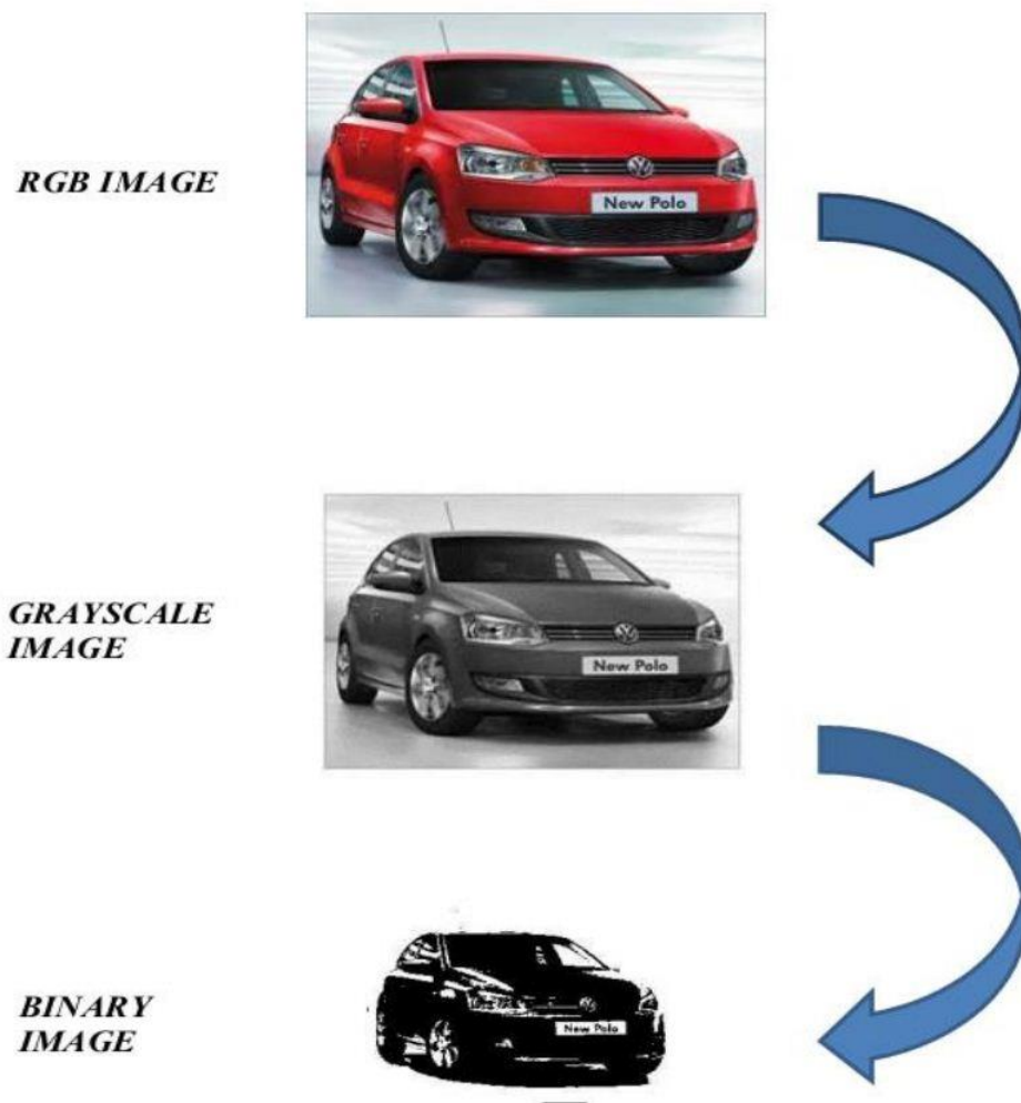
Figure 1. 4 Conversion from RGB Image to GRAY Image, GRAY Image to Binary image
