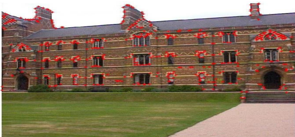
Figure 2.3. Image with corner feature using Harris Corner detection algorithm.
