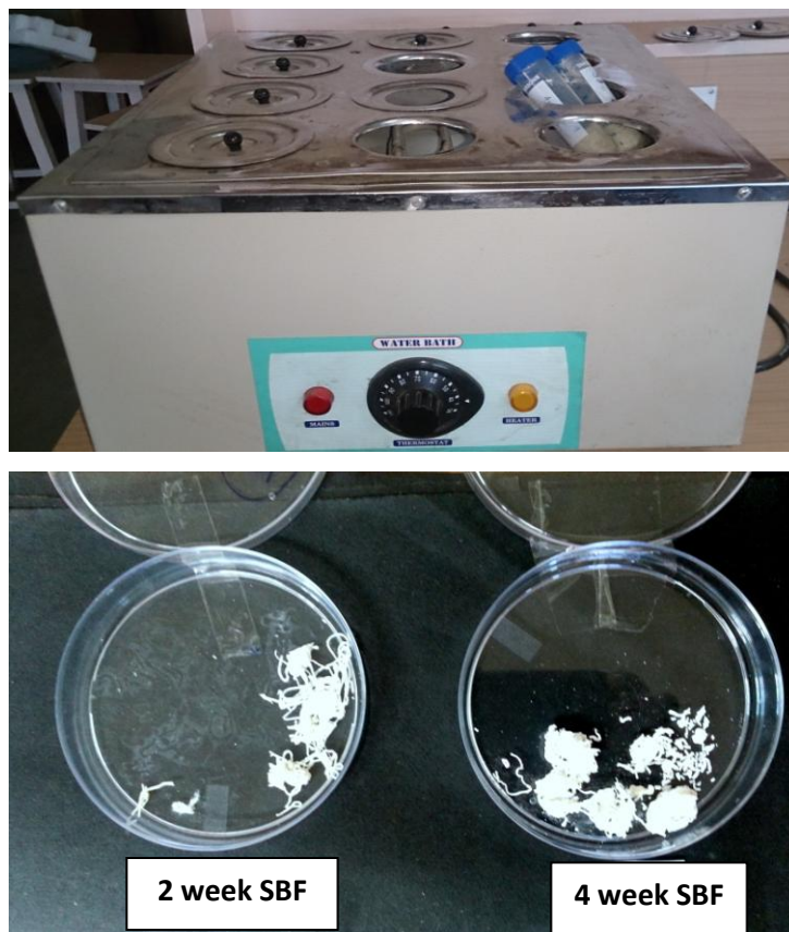
Figure 9: (a) Samples maintained in 37°C in SBF for 2 weeks and 4 weeks, (b) Dried samples after immersion in SBF for 2 weeks and 4 weeks
