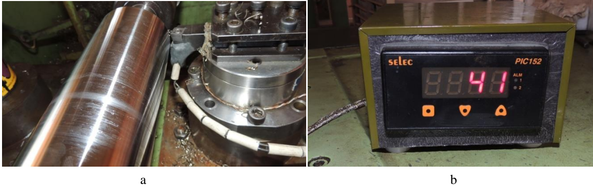
Fig. 15 Temperature measurement set-up a) Thermocouple b) Temperature recorder
