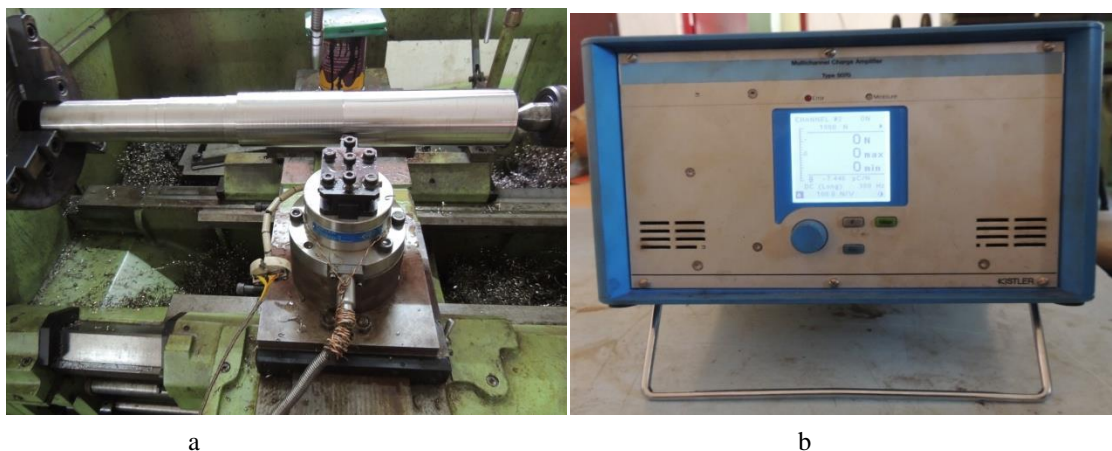
Fig. 14 Cutting force set-up a) dynamometer b) charge amplifier
