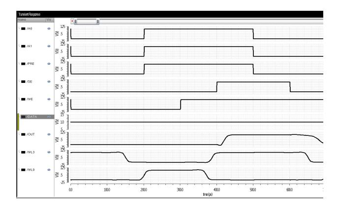
In read operation when both the inputs gets low at that time data is being kept at the constant value. When w13 goes from high to low and w10 goes from low to high with sense enable gets on we get confirmed for the read operation of the memory cell.
