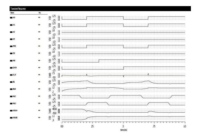
In write operation when the write enable gets on after that the data goes high from low to high after that remains constant, which shows that the data is being read by the memory cell.
