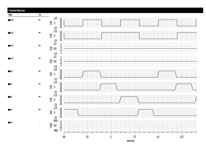
The output follows the input but after some interval of time. Because of the delay in the design i.e 270 ps. So we are getting the desired output after some intervals. We need to minimize these interval inorder to get some specification.
