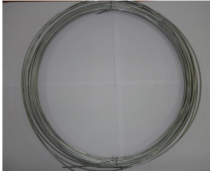
Figure3.1: GI wires (used for making the inserts)
