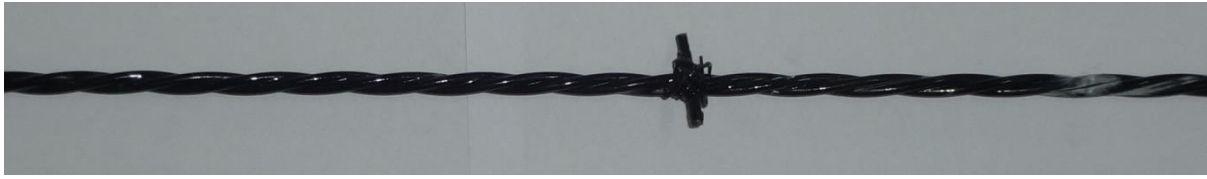
Fig 3.3b: Insert made up of three GI wires
