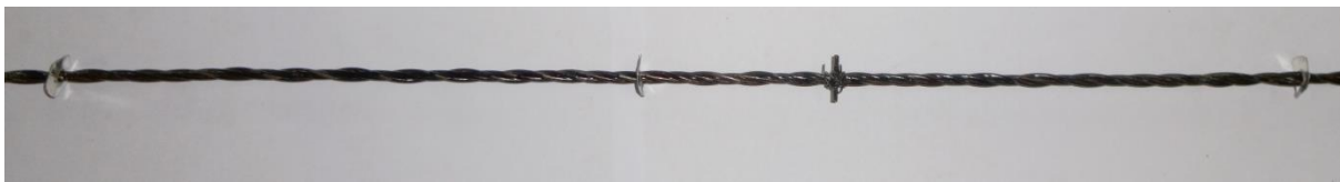
Fig3.3d: 3 wire insert with \beta= 24\text{cm}
