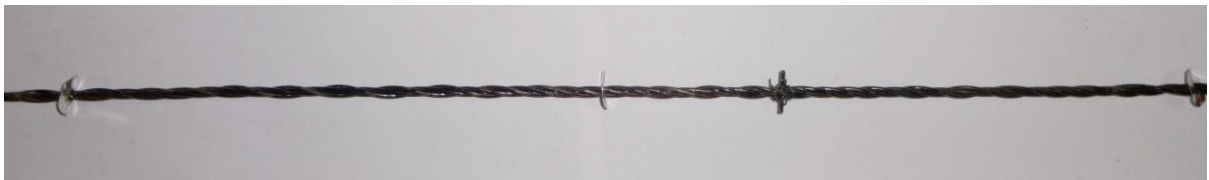
Fig3.3f: 3 wire insert with \beta= 6\text{cm}
