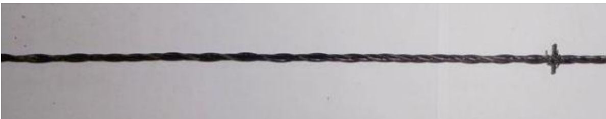
Figure 4: 4 wire insert without baffles
