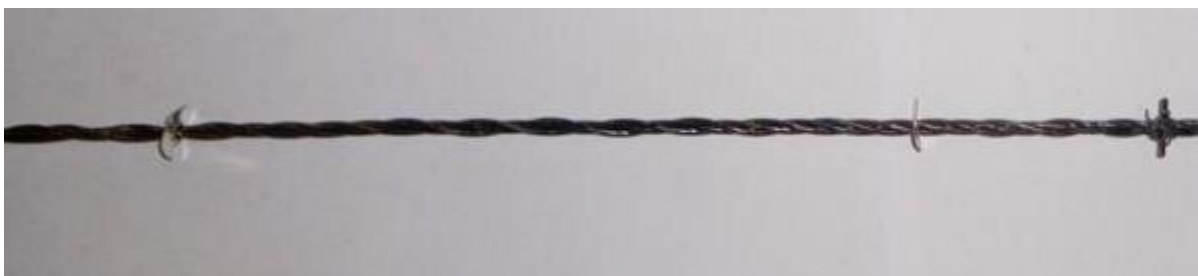
Figure 6: The 4 wire insert with baffle spacing 24cm
