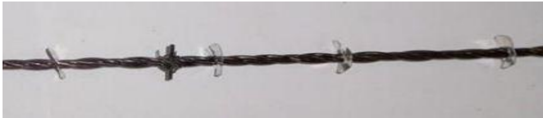
Figure 8: 4 wire insert with baffle spacing 6cm.
