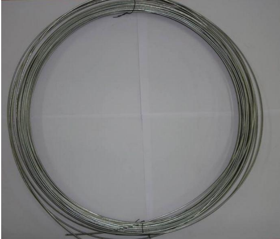
Figure 3: Galvanised Iron wire used to make the insert.
