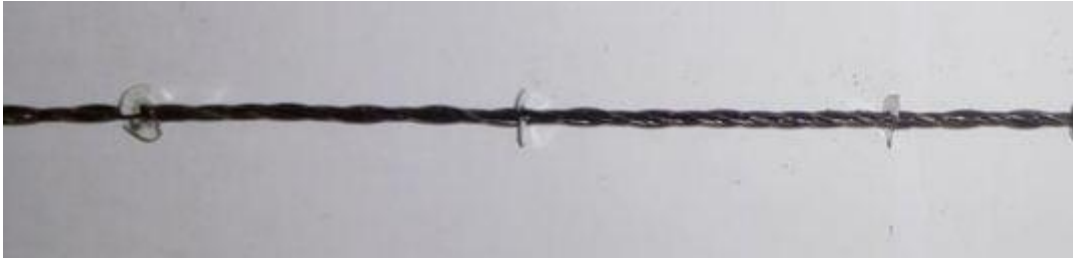
Figure 7: 4 wire insert with baffle spacing 12cm.
