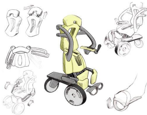
Figure 9. Mechanism for seat lifting [6]
