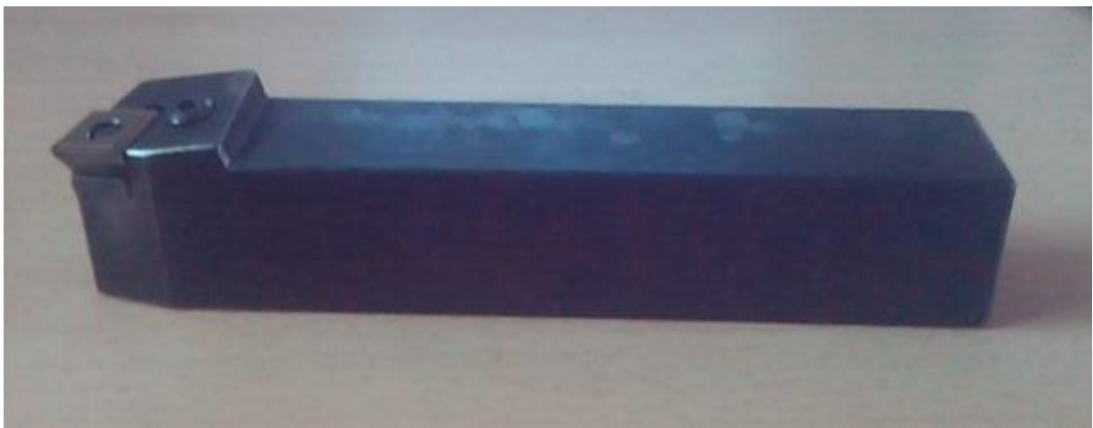
Fig-4.3:Tool holder (PSBNR2525M12)
