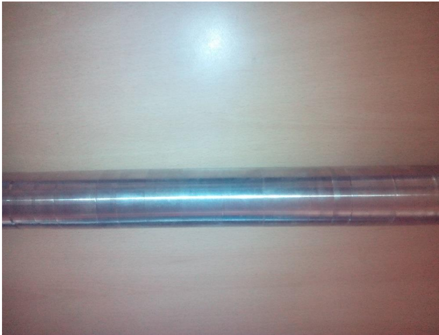
Fig-4.1: Work piece material(Cr-Mo round bar)
