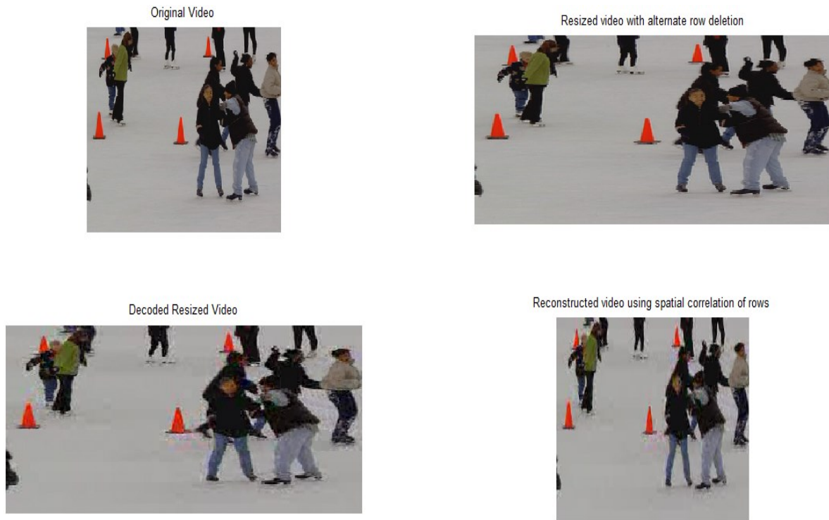
Fig.7. 9: Frame 10 of Ice_cif video and its resized, decoded and reconstructed frames using spatial correlation of rows
