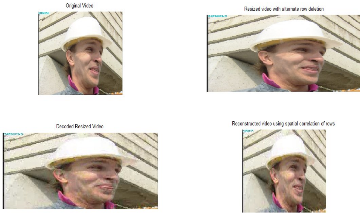
Fig.7. 7: Frame 10 of Foreman_cif video and its resized, decoded and reconstructed frames using spatial correlation of rows
