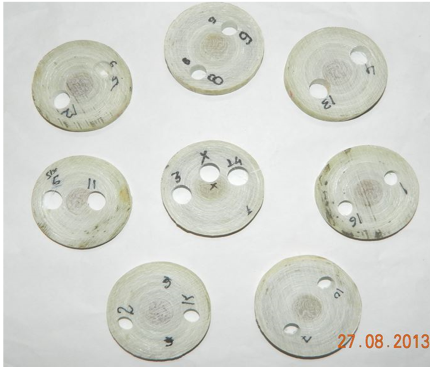
Fig. 2.3: GFRP epoxy work pieces after machining
