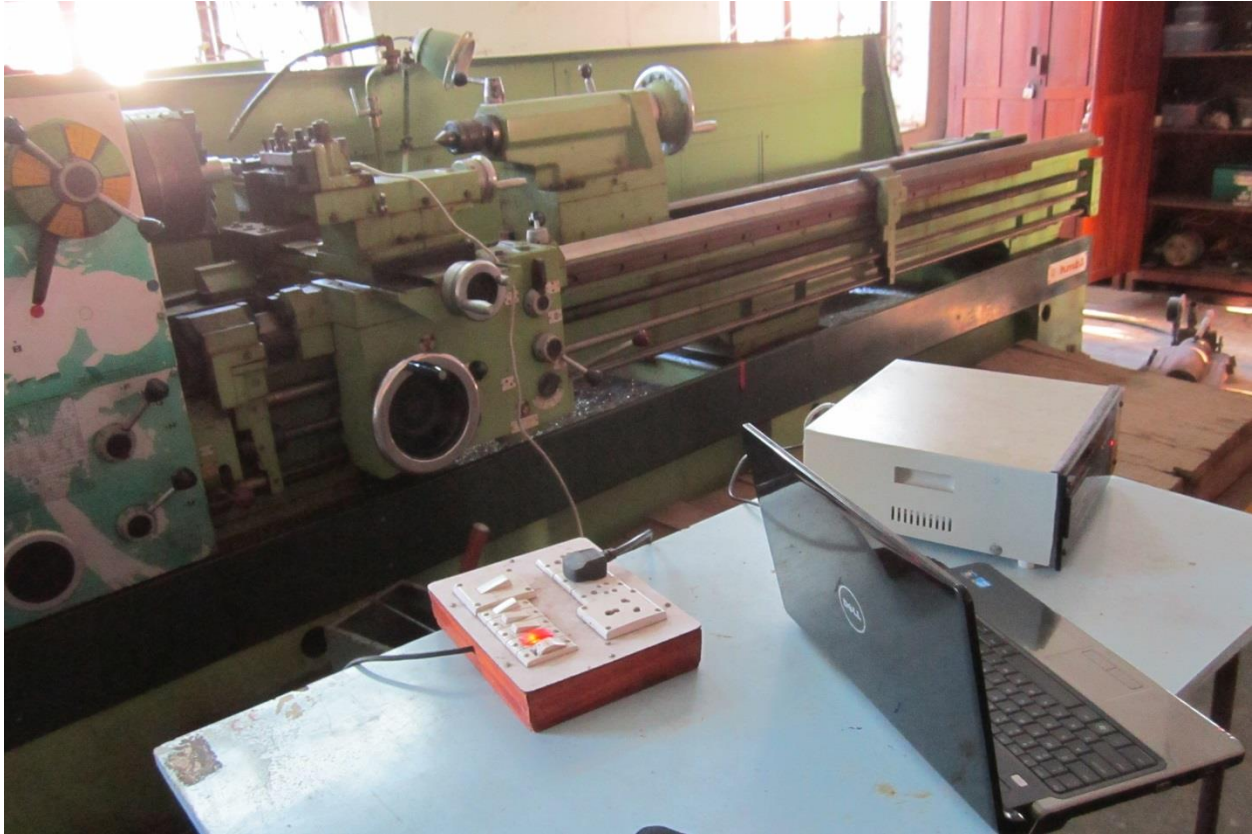
Fig 6: Experimental setup with computerized dynamometer
