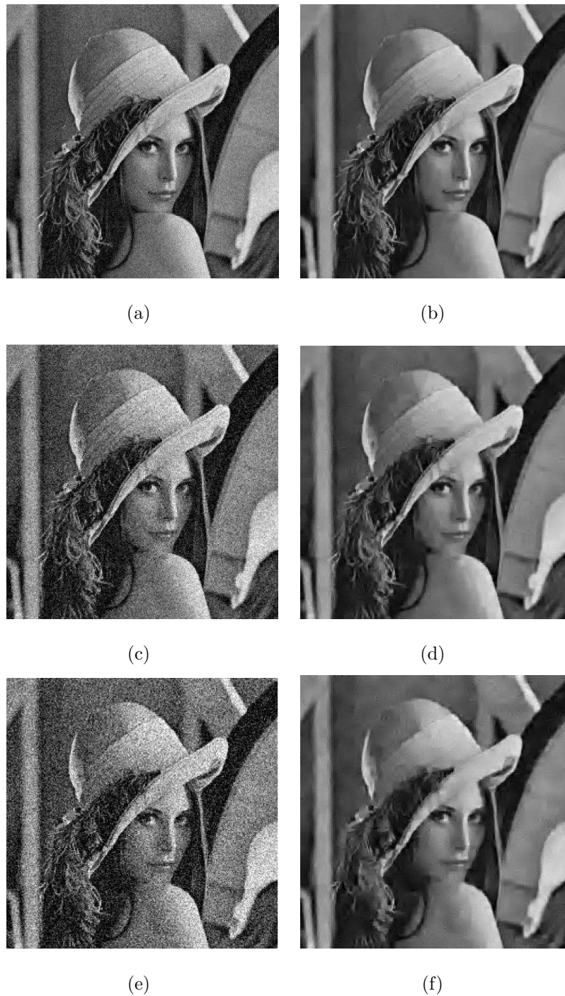
Figure 3.6: Denoised Lena images(a) Noisy Lena Image ( \sigma = 10 ) (c) Noisy Lena Image ( \sigma = 20 ) (e) Noisy Lena Image ( \sigma = 30 ) (b),(d),(f) Denoised Images by Proposed Method.
