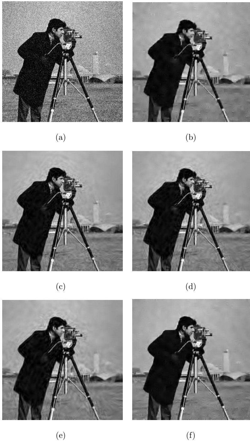
Figure 3.5: (a) Cameraman Image with noise level ( \sigma = 20 ) (b) Denoised using neighshrink (26.44db) (c) Denoised using Bivariate (30.23db) (d) Denoised using GIDNWC (27.42db) (e) Denoised using IAWDMBNC (27.76db) (f) Denoised using MLMMSE (30.40db) .
