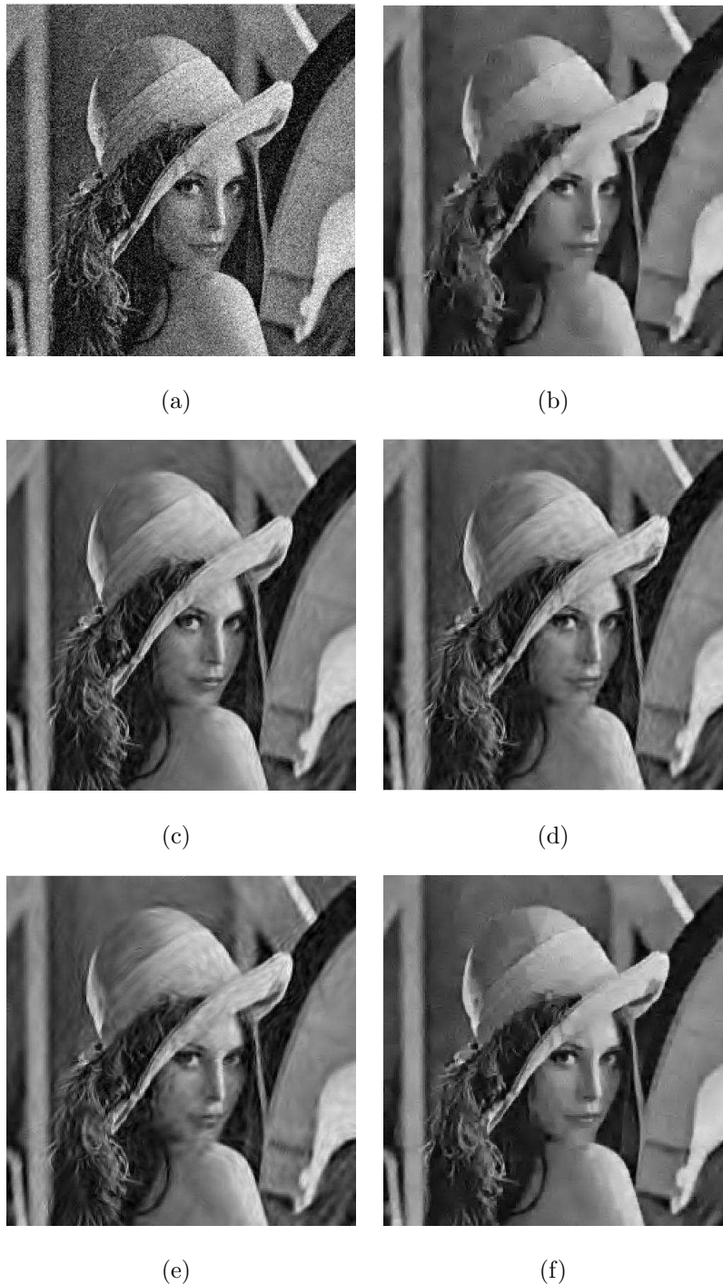
Figure 3.4: (a) Noisy Lena with ( \sigma = 20 ) (b) Denoised using neighshrink (28.56db) (c)Denoised using Bivariate (30.50db) (d) Denoised using GIDNWC (29.22db) (e)Denoised using IAWDMBNC (29.56db) (f)Denoised Image using MLMMSE (30.74db) .
