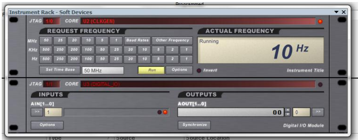
Fig 4.2.2:- The frequency generator
