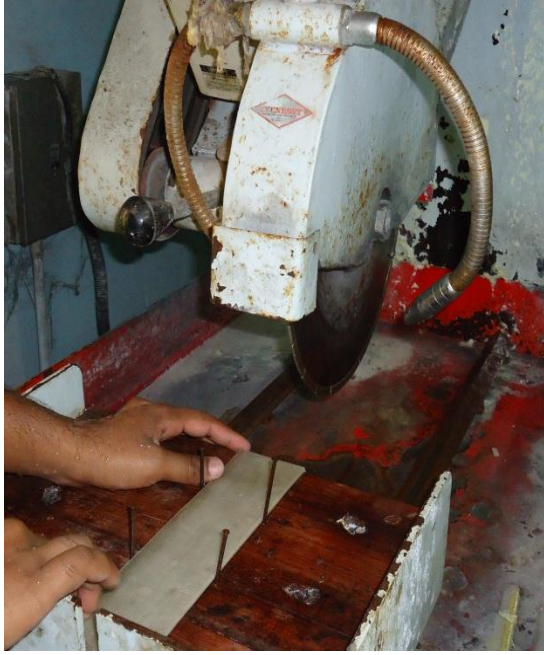
Fig 4: Diamond cutter for cutting specimens
