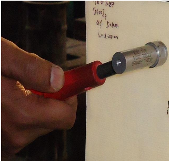
Fig 18: Modal Impact Hammer (type 2302-5)
