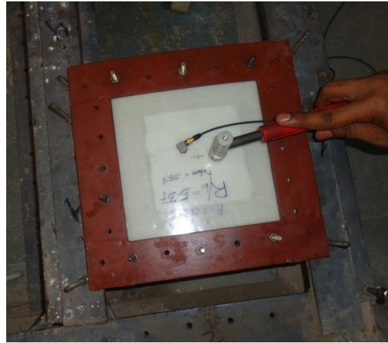
Fig 16: Frame for C-C-C-C boundary condition.
