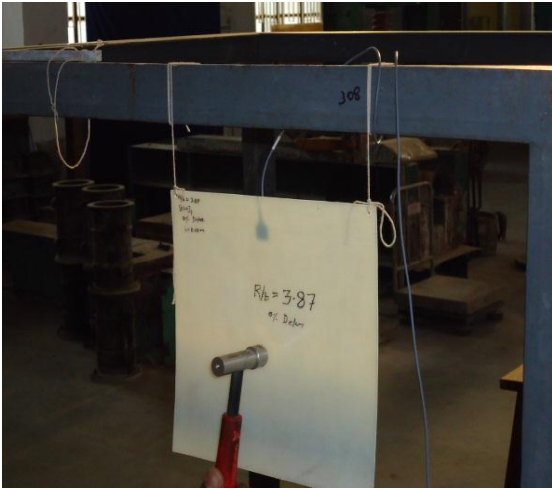
Fig 15: Frame for F-F-F-F boundary condition.
