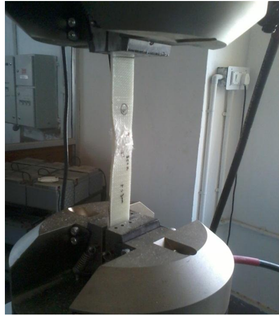
Fig 7: WR glass/epoxy specimen during tensile testing
