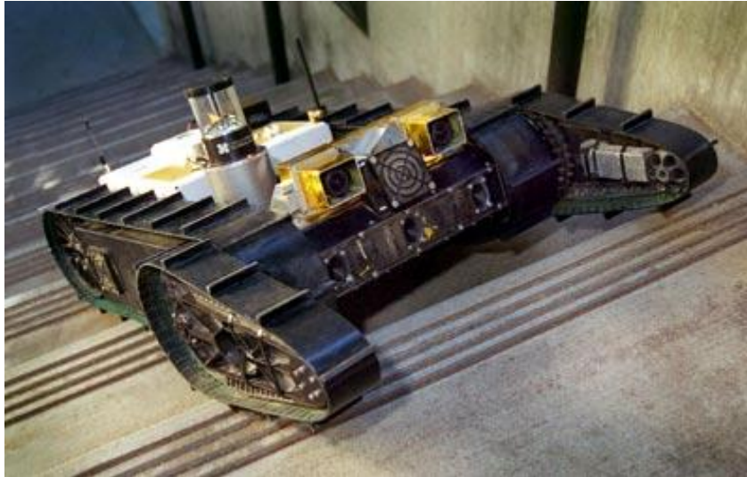
Figure 2.1 Autonomous Urbie developed by NASA, is designed for various urban operations, including military reconnaissance and rescue operations.
