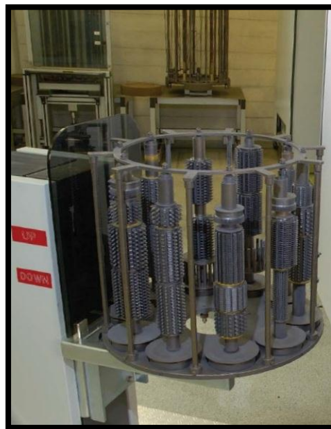
Figure 10. RCS system for coating deposition(Source : Oerlikon Balzer)
