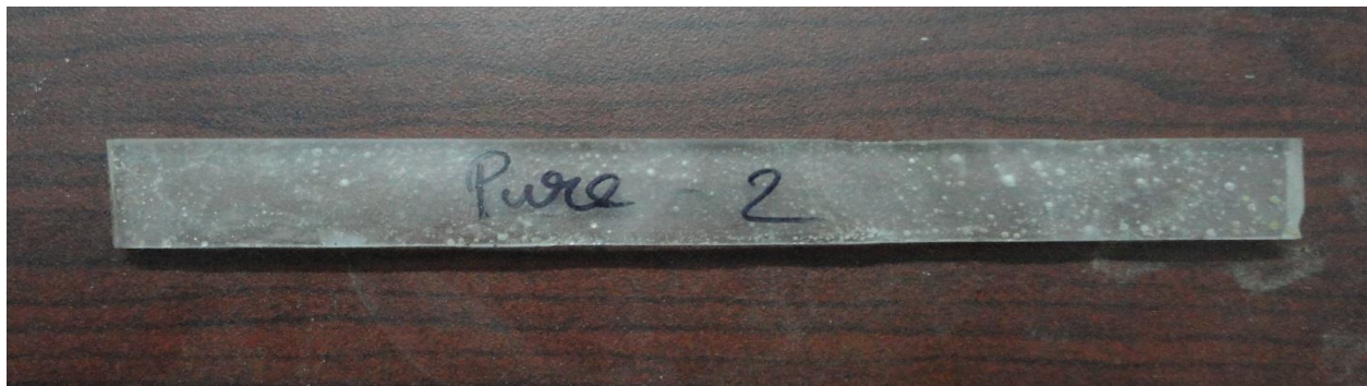
Fig 4.2 Three point bending test sample/flexural test sample
