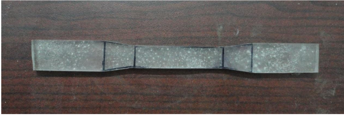
Fig 4.10 Dog bone shaped specimen for tensile test
