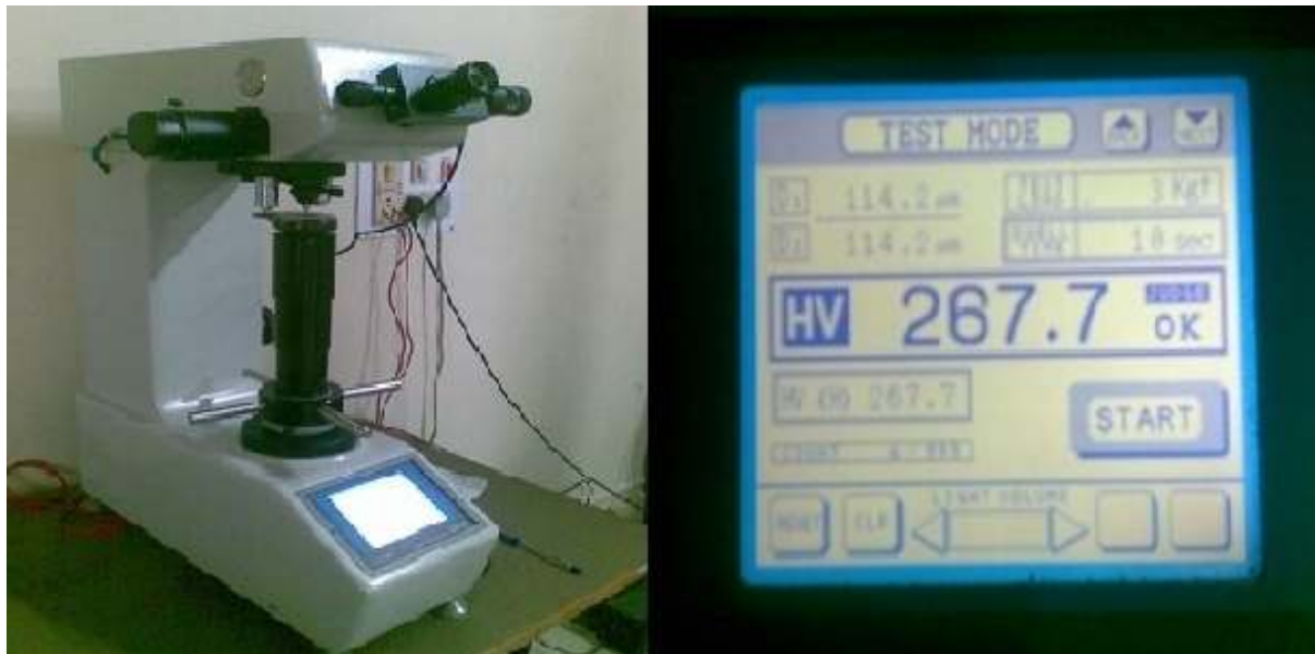
Fig. 17: (a) Vickers hardness machine (b) Data acquisition system
