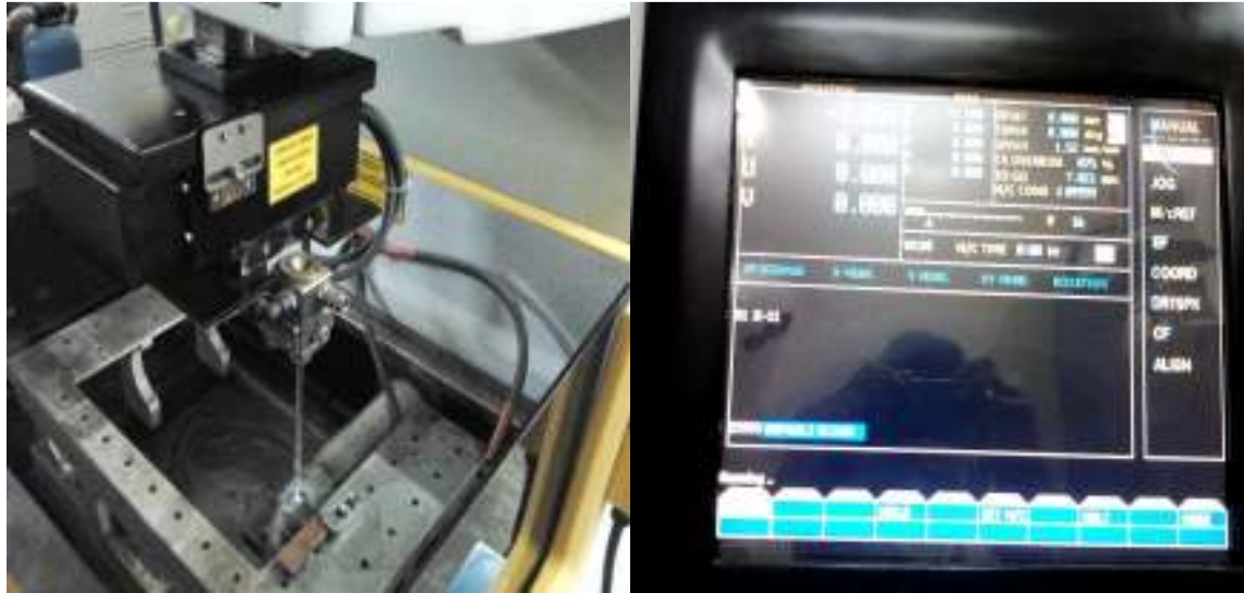
Fig. 18: (a) Cutting samples by WEDM (b) Data acquisition system
