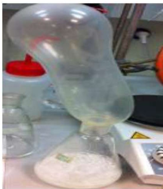
Figure 7 CO 2 absorbed is easily separated by heating
