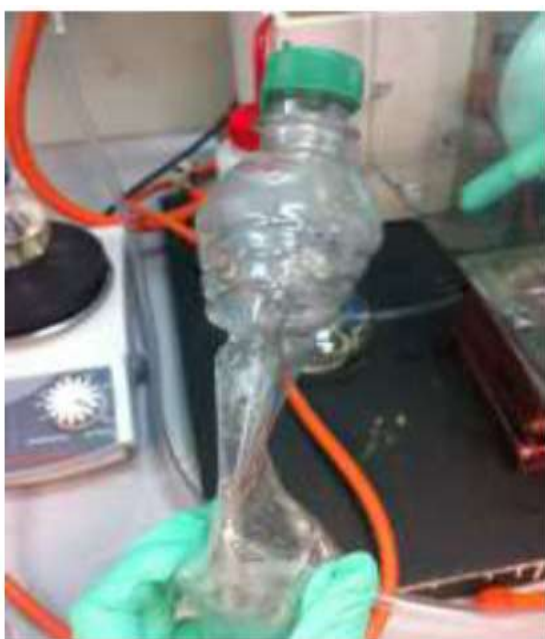
Figure 6 Experiment to show MEA captures CO 2
