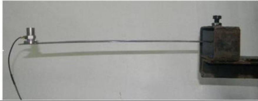
Fig 20: Experimental setup for a cantilever beam
