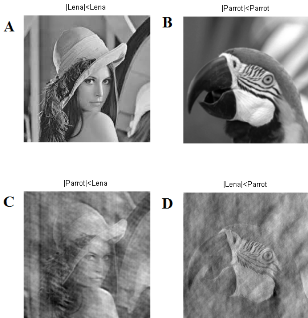
FIGURE 2.1: Phase vs Magnitude. A - Lena image. B - Parrot image. C - IFFT of Phase from A and Magnitude from B. D - IFFT of Phase from B and Magnitude from A.
