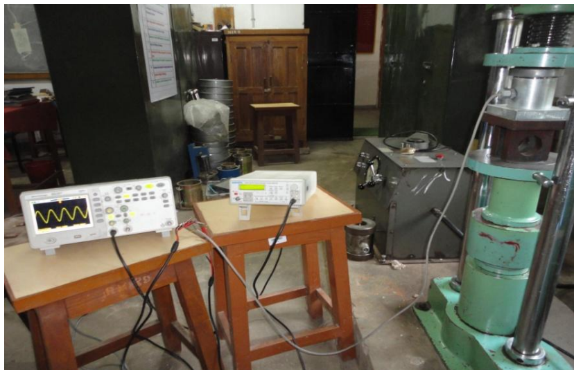
Fig 3.1 Experimental setup for determination of the optimum output frequency range
