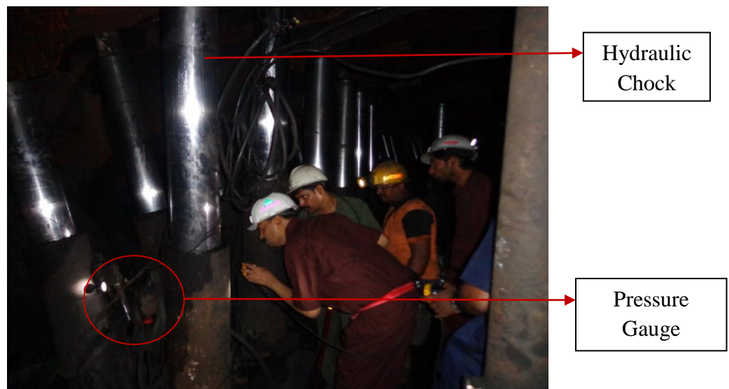
Fig 1.3 Hydraulic chock shield with inbuilt pressure gauge[2]
