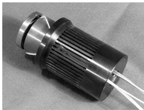
Figure 4. The smart actuator integrated into the mechatronic module.
