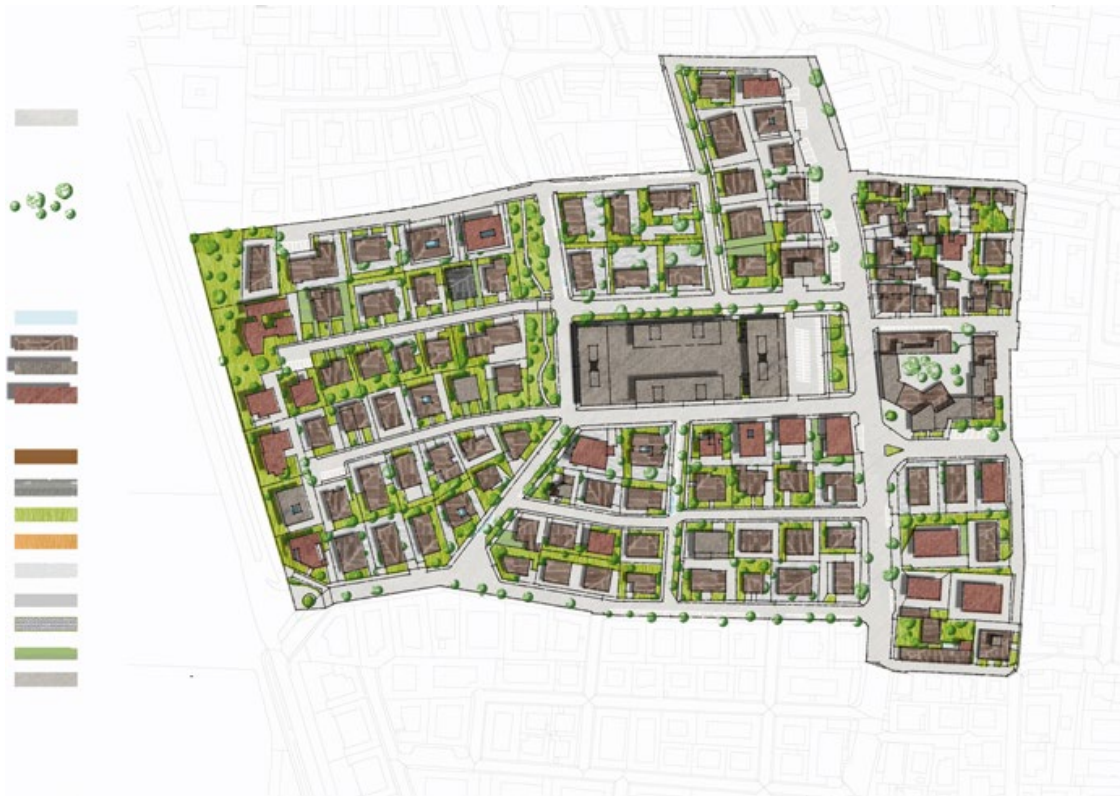
Fig. 8.13 Intervention 4 + summary of intervention 4 Albedo on private paved surfaces. Modify the reflectance on private surfaces
