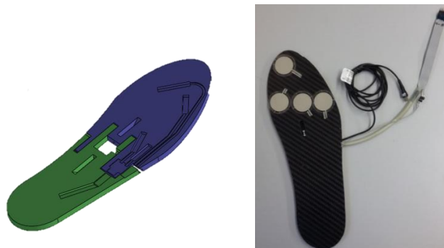
Fig. 1 The CAD model and the prototype of the sole with some piezo-resistive sensors and the I/O apparatus
