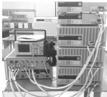
Figure 3. A test bench with electronic loads.
