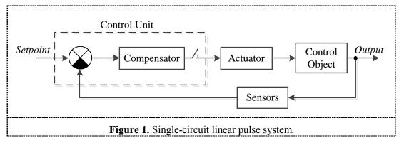
Single-circuit PCS can be presented as a combination of digital and continuous subsystems interacting with each other. The continuous part contains a control object as well as intensifying and executive devices [4,6]. The digital part, as a rule, is the control device and integrates the functional elements participating in impulse transformation of a signal.
