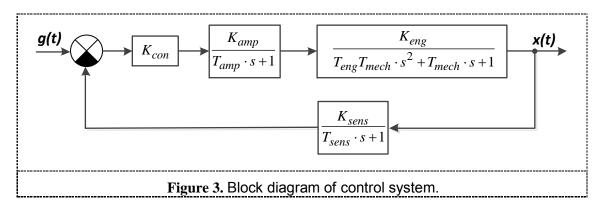
As it was noted earlier, an essential analysis stage is obtaining of impulse TF of open-loop system  $W_{loop}(z)$ . For this purpose, one can use the Control System Toolbox module containing a necessary set of functions.
