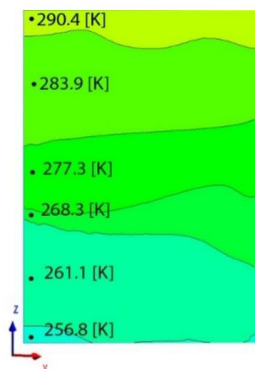
Fig. 2. Temperature field distribution at the exit area.
