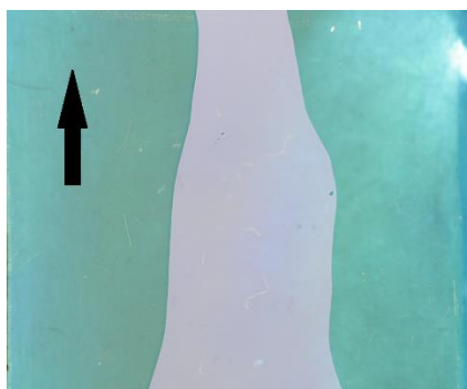
Fig. 6. The nitrogen driven water rivulet flow regime in the minichannel-rivulet bridge.
