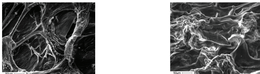
FIGURE 2. SEM image of the Orgamax OPM surface (sample TVCH 1060) made of DMBC
