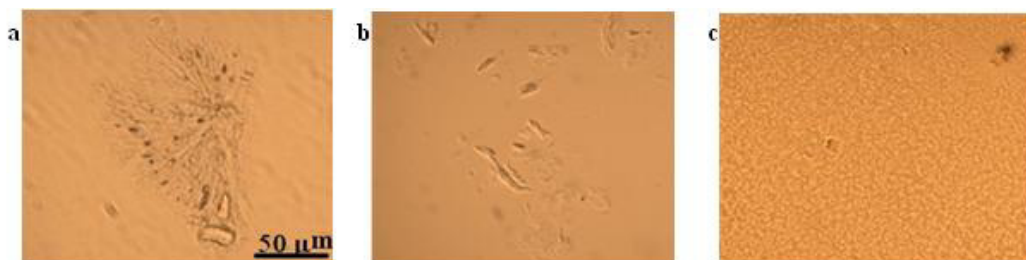
Fig. 6. (a) GK1; (b) 0.5 % oil; (c) 2 % oil micrographs of OGKM deposits based on GK1 with addition of oil
