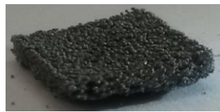
Figure 12. Physical configuration of a three-dimensional sample (x2). Process conditions of sintering: V=1000 mm/min, t=26 °C, S=0.1 mm, P=60 W, increment thickness of layers 200 \mu\text{m} , sintering in argon
