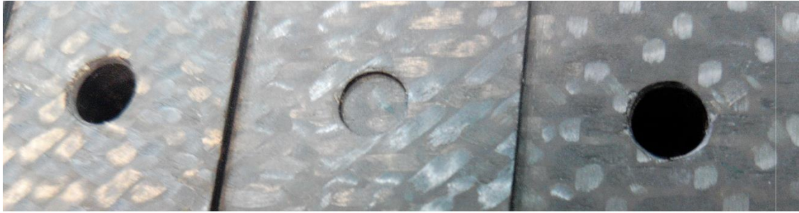
Figure 4. Flat-bottom holes on the reference sample.
