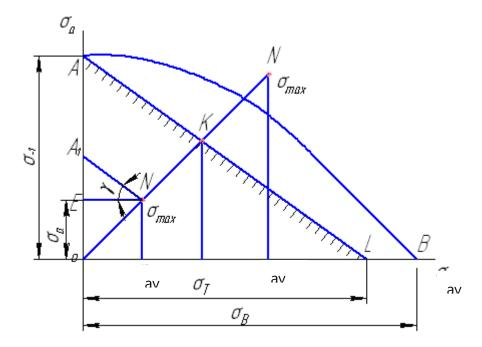
Fig.1. Schematized diagram of limiting amplitudes
