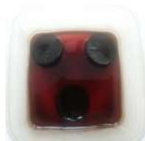
Figure 4. Darkening of diesel fuel under temperature influences (100° C) on elastomer's samples
