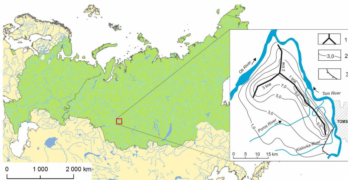
Figure 1. Layout of Tomsk water intake facilities: 1-production well line of water intake facility; 2 – contours of decreasing groundwater level, m; 3 – Paleozoic basement protusion borderline.
