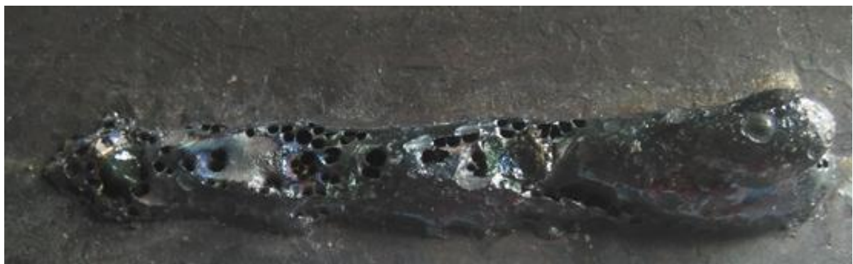
Figure 3 – Quality of the weld surface with a 5–10 mm fraction used in welding
