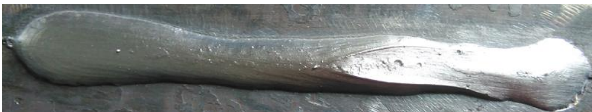
Figure 4 – Quality of the weld surface with a fraction of less than 0,45mm used in welding
