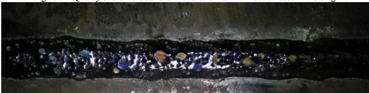
Figure 2 – Quality of the weld surface with a 2.5–5 mm fraction used in welding
