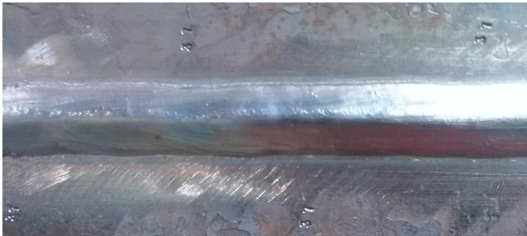
Figure 1 – Quality of the weld surface with a 0.45–2.5 mm fraction used in welding
