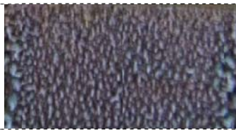
Figure 49. External appearance of sintered surface PMS-1 (x2). Process conditions: P=30W, V=200 mm/min, S=0.1 mm, t=26 °C, non-activated.
