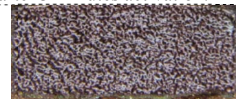
Figure 54. External appearance of sintered surface PMS-1 (x2). Process conditions: P=22 W, V=160 mm/min, S=0.2 mm, t=26 °C, after 3 minutes activation.
