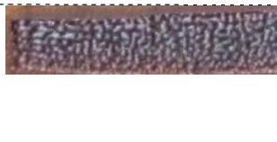
Figure 43. External appearance of PMS-1 surface (x2). Process conditions: P=30 W, V=3000 mm/min, S=0.1 mm, t=200 °C, non-activated.
