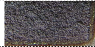
Figure 48. External appearance of PMS-1 surface (x2). Process conditions: P=15 W, V=3000 mm/min, S=0.1 mm, t=200 °C, after 3 minutes activation.
