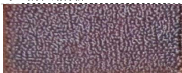
Figure 53. External appearance of sintered surface PMS-1 (x2). Process conditions: P=22 W, V=160 mm/min, S=0.2 mm, t=26 °C, non-activated.
