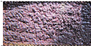
Figure 41. External appearance of PMS-1 surface (x2). Process conditions: P=15 W, V=200 mm/min, S=0.3 mm, t=26 °C, after 1 minute activation
