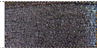
Figure 42. External appearance of PMS-1 surface (x2). Process conditions: P=15 W, V=200 mm/min, S=0.3 mm, t=26 °C, after 3 minutes activation.
