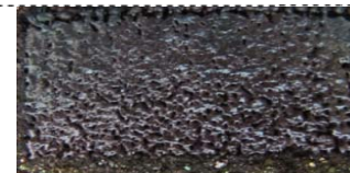
Figure 45. External appearance of PMS-1 surface (x2). Process conditions: P=30 W, V=3000 mm/min, S=0.1 mm, t=200 °C, after 3 minutes activation.
