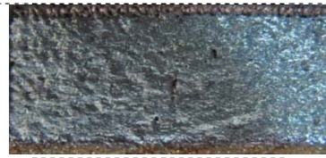
Figure 52. External appearance of sintered surface PMS-1 (x2). Process conditions: P=15 W, V=200 mm/min, S=0.1 mm, t=26 °C, after 3 minutes activation.
