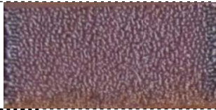
Figure 35. External appearance of PMS-1 surface (x2). Process conditions: P=30 W, V=3000 mm/min, S=0.3 mm, t=26 °C, non-activated.
