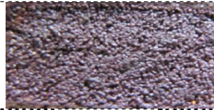
Figure 47. External appearance of PMS-1 surface (x2). Process conditions: P=15 W, V=3000 mm/min, S=0.1 mm, t=200 °C, after 1 minute activation
