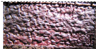
Figure 44. External appearance of PMS-1 surface (x2). Process conditions: P=30 W, V=3000 mm/min, S=0.1 mm, t=200 °C, after 1 minute activation
