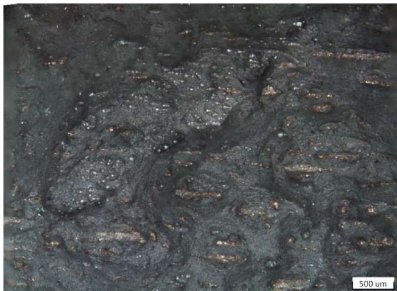
Figure 2. Kind of fracture of the sample with lowered plastic properties, selected products 2A82-1M
