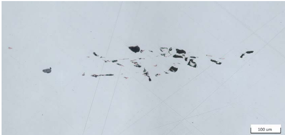
Figure 3. Specific inclusion in the metal sample, № R6986A1-1 view of the micro section
