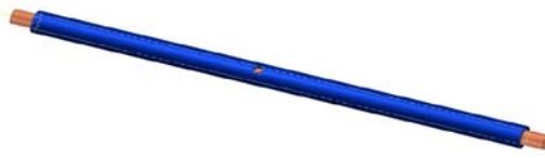
Figure 3. Example of a through defect.
