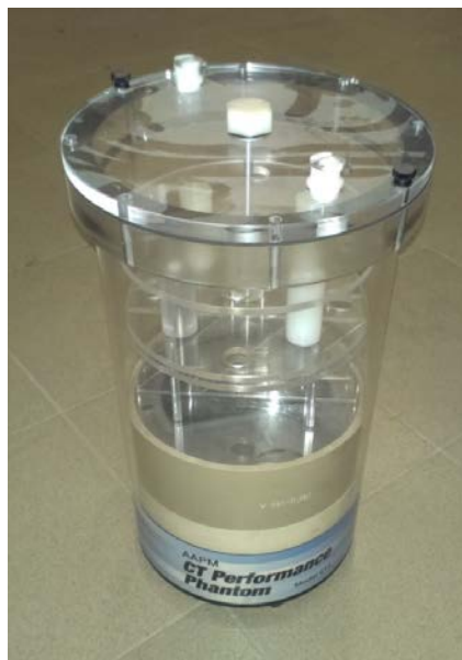
Figure 4. The exterior of AAPM CT Performance Phantom, model 610.
