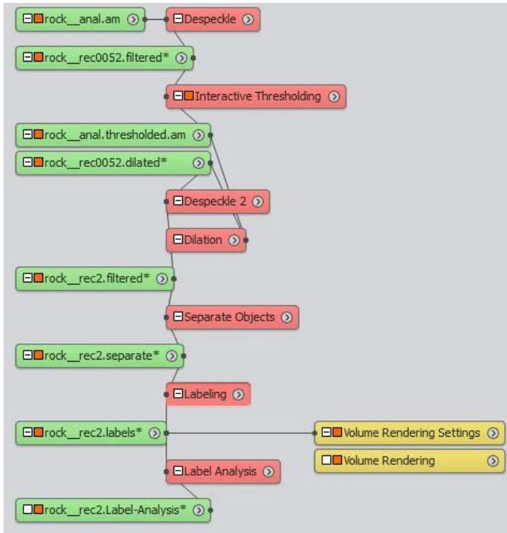
Figure 4. The scheme of image processing applied to gravel mixture from despeckle step to quantitative analysis.
