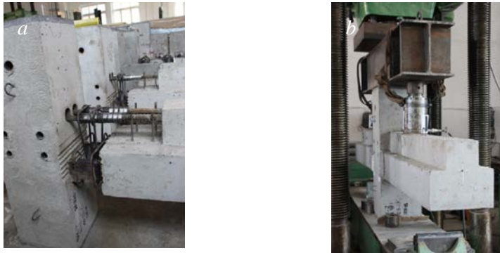
Figure 9. General view of beam-to-column connection: a – mechanical coupler; b – static load test.
