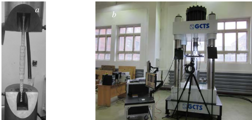
Figure 3. Photographs of load tests: a – tensile load test on Tensile Testing Machine MR-500; b – compressive load test on the Universal Testing Machine 4500.
