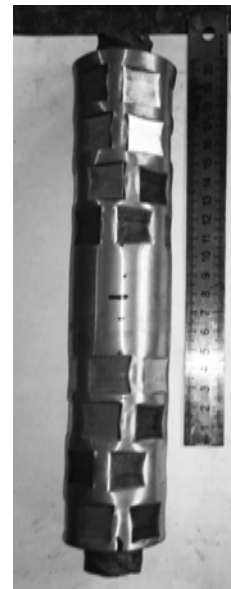
Figure 2. Photograph of mechanical rebar splice.
