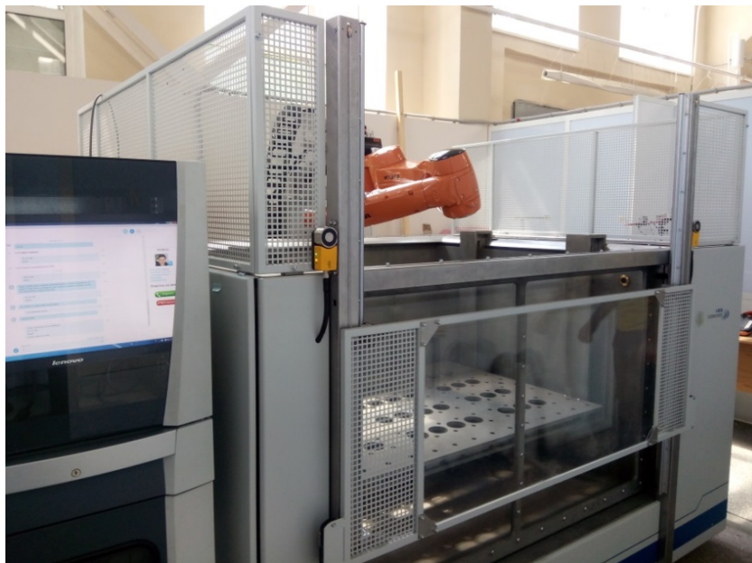
Figure 1. Complex of ultrasonic inspection.
