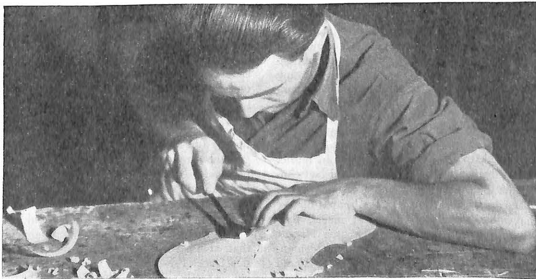
Shaping the back of a violin. The instrument does not acquire its curve by bending; it is, as a 17th century English maker put it, "dugged out of the planke."
