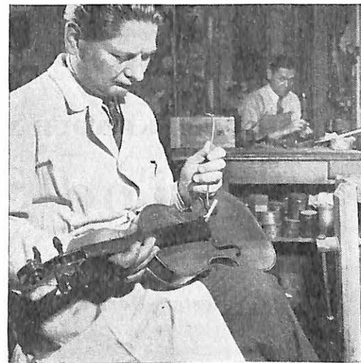
Inserting the soundpost is a very tricky operation, and requires the deft fingers of a skilled craftsman.
